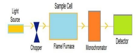
Fig. 3: Schematic Diagram of AAS (Csuros, M., Csuros, C., 2002)
